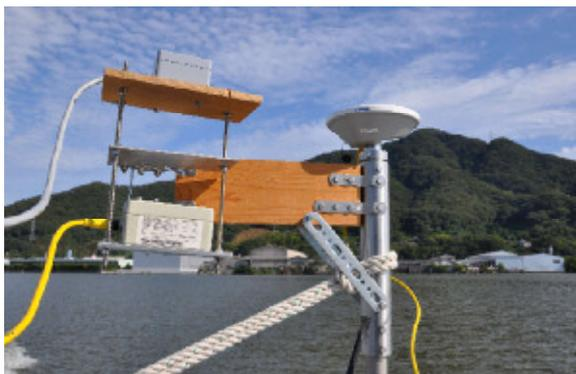
(a) A GPS antenna attached to one end of a pole.
