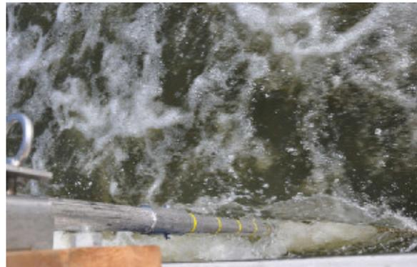
(b) An oscillator of an echo sounder was attached to the other end of the pole beneath the water surface.
